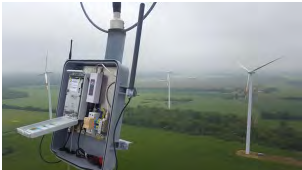
LoRaWAN IoT network deployment by Raycap, using Kerlink Wirnet Station gateway
