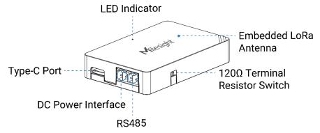
**120\Omega Terminal Resistor Switch**: the device will add a 120 $\Omega$  termination resistor to avoid data-corrupting reflections if RS485 data rate is high or cable length is long.
