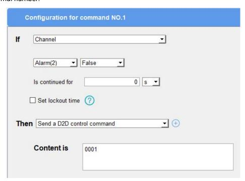
When UC100 receives a Milesight D2D command, it can work as a Milesight D2D agent to reboot the device, send a LoRaWAN® message or send Modbus command to RS485 terminal devices.
