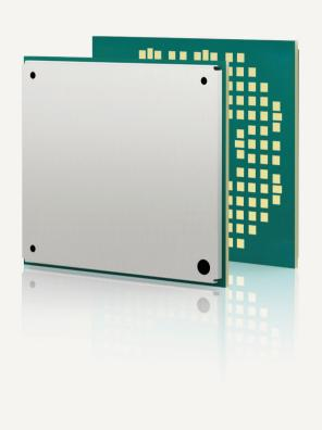
Cinterion® PLS8 Wireless Module Best In Class LTE Connectivity for the Industrial IoT
