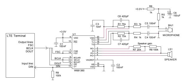
Figure 13: Sample circuit for analog to DAI/PCM circuit
