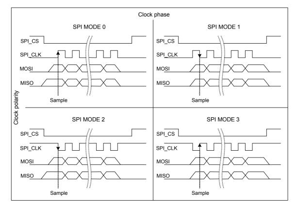
Figure 15 shows the characteristics of the four SPI modes. The SPI modes 0 and 3 are the most common used modes.
