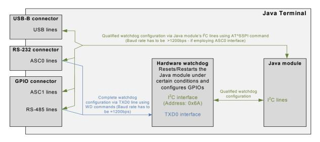
Figure 26: Hardware watchdog configuration
