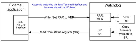
Figure 28: Read data from address register
