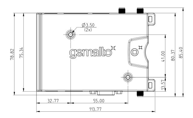
Figure 22: LTE Terminals mechanical dimensions
