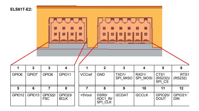
Figure 9: ELS61T-E2: GPIO connectors (8-pin and 12-pin)
