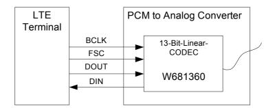
Figure 12: Block circuit for DAI/PCM to analog converter
