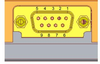
Figure 7: Pin assignment RS-232 (D-sub 9-pole female)
