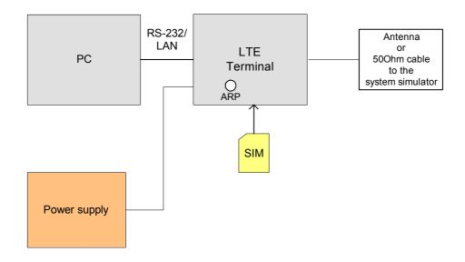
Figure 25: Reference equipment for approval
