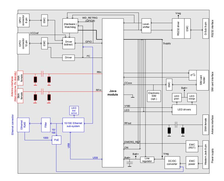
Figure 6: LTE Terminals circuit block diagram
