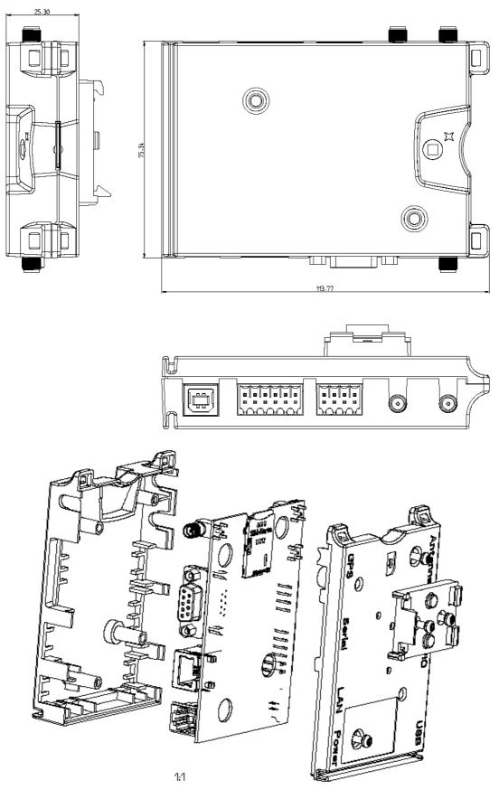
Figure 23: LTE Terminals exploded view
