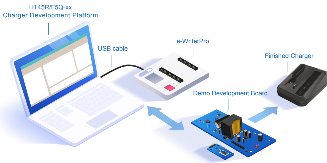
Figure 4. Holtek Charger Development Platform Development Process
