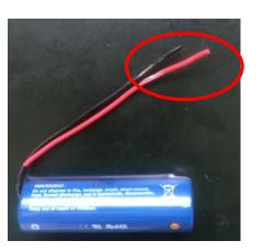
Make sure the naked battery or wire will not contact PCB
