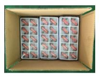
◆ The batteries shall be insulated and separated, preferably to be placed in the original trays. The trays shall be bundled up with tapes and be loaded into cartons. Fill the space with foam or carton boards inside the carton to fix the trays.
