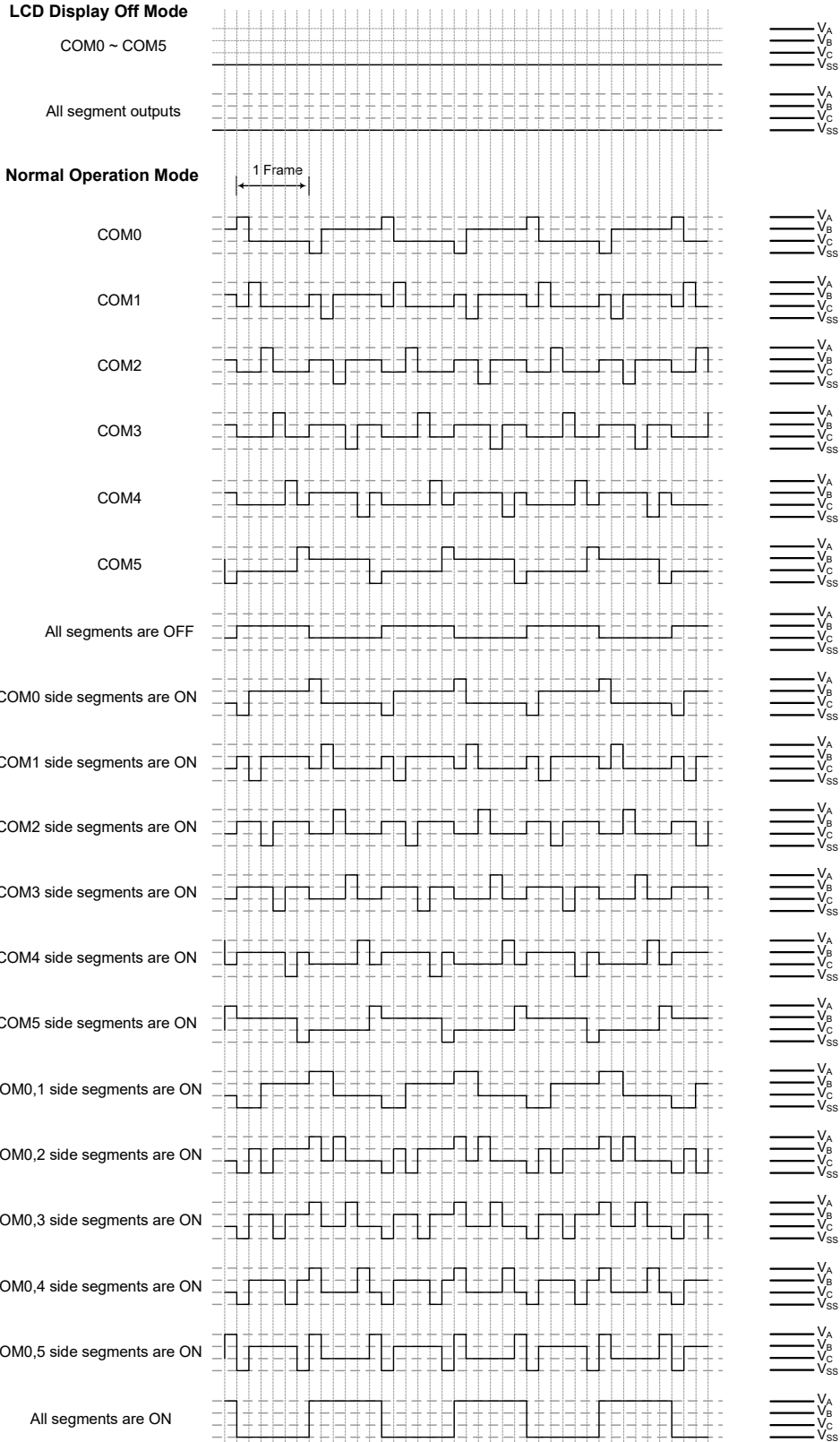
LCD Driver Output – Type B, 1/6 Duty, 1/3 Bias
