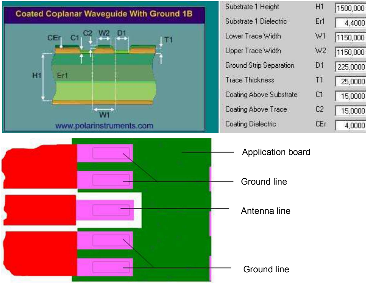
Figure 44: Micro-Stripline on 1.5mm Standard FR4 PCB - example 2
