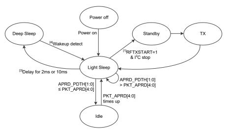
Note: 1. Once the RFTXSTART control bit is enabled, the I<sup>2</sup>C will stop and the RF chip will start transmiting data.
