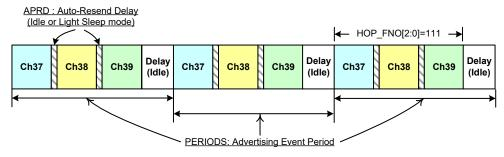
PKT\_APRD[4:0]: Packet format auto-resend delay, 250µs (Min.) ~ 8ms (Max.)
