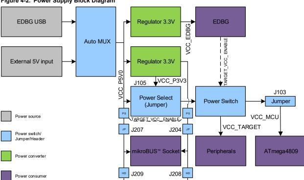
Figure 4-2. Power Supply Block Diagram
