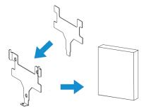
2. Put the device on the mounting bracket, then fix the bottom of the device to the bracket with the theft-deterring screw.
