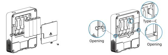
3. Fix the rear cover back to device with the fixing screw.
